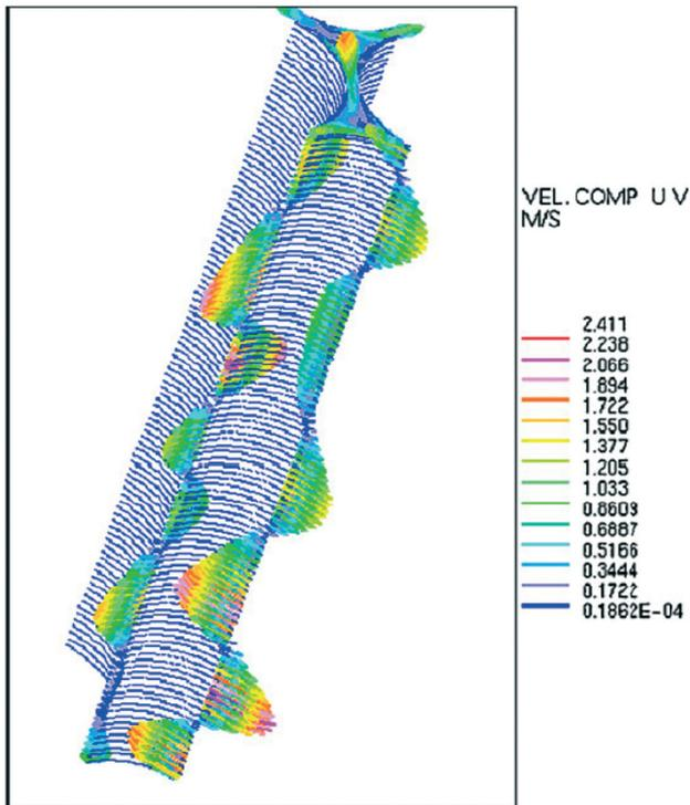
Fig. 6 Flow oscillation between subchannels and cross flow velocity components.
