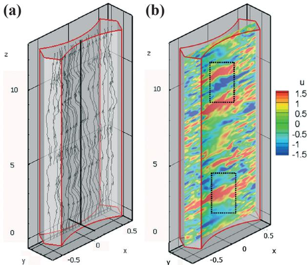
Fig. 5 (a) Streamlines (b) Contour plot for the instantaneous cross flow velocity in an infinite triangular lattice rod bundle  $P/D=1.05$ ,  $Re=5,500$ .
