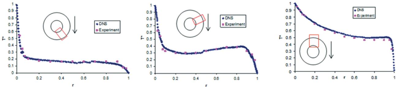
Fig. 2 Radial temperature distributions at different angle positions in the concentric annulus: comparisons of DNS and experiment.
