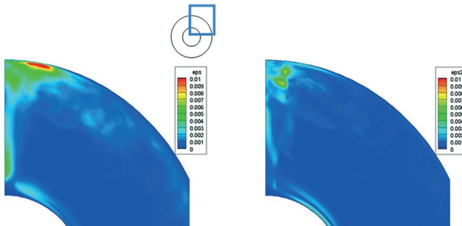
Fig. 3 SGS dissipation: DNS filtered (left) and Dynamic Smagorinsky (right).
