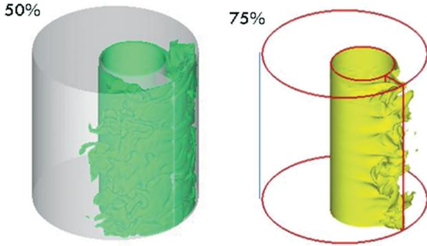
Fig. 4 Normalized temperature ( $T^* = (T - T_{out}) / (T_{out} - T_{in})$ ) contours in an eccentric channel:  $T^* = 0.5$  (left) and  $T^* = 0.75$  (right).
