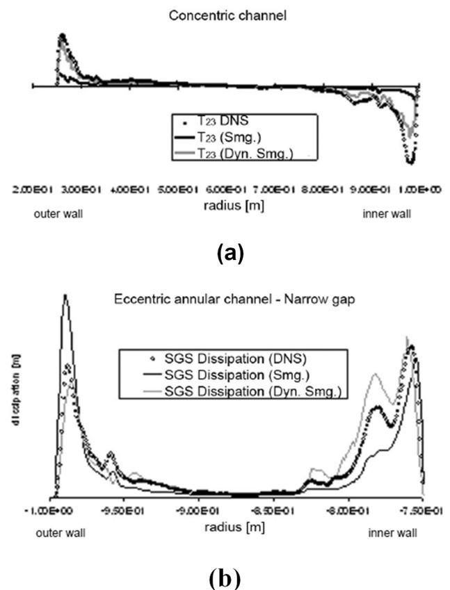
Fig. 1 A priori test for concentric and eccentric channels. Direct comparison for the stresses (a) and comparison for the SGS dissipation (b).
