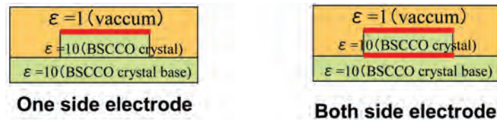
Fig. 9 Affection of electrode configuration on Josephson plasma excitation.
