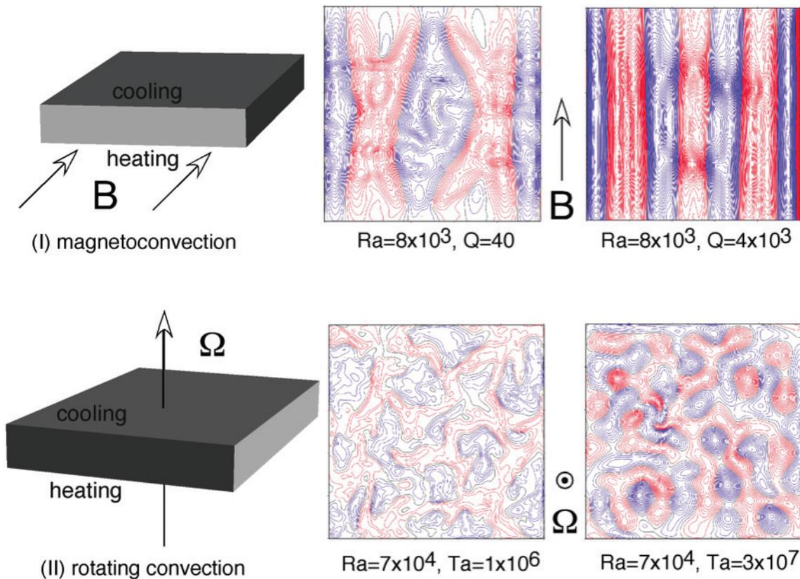
Fig. 4 Setting and result of numerical simulations. (I) Convection under uniform horizontal magnetic field. (II) Convection on a rotating system.  $Pr$  of the fluid is 0.025. The contours are flow velocity in vertical direction; red indicates the upward flow, and blue indicates downward flow. In (I), the flow pattern is restricted to be rolls in the direction of magnetic field for larger  $Q$ . In (II), the pattern is composed of vortices and gets shorter for larger  $Ta$ .
