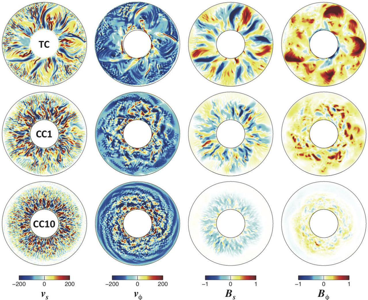
Fig. 3 The convective structures of our TC model of  $Pr = 1$  (top), CC model of  $Pr = 1$  (middle), and CC model of  $Pr = 10$  (bottom). From left to right, the cylindrically radial and the azimuthal velocities, the radial and the azimuthal magnetic fields are shown at  $z = 0.1$ . The TC model is identical to our previous UHF model [5]. In the CC model, the reference temperature gradient is assumed to be proportional to  $r - 1/r^2$ , where  $r$  is the radius normalized by the core radius.
