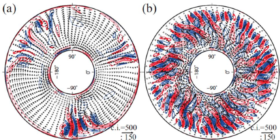
Fig. 1 Snapshot of convection structure on the plane at  $z = 0.2$  viewed from the north, where  $z$  is the distance from the equatorial plane. Cases for dynamo (a) and purely thermal convection (b) are shown. The axial component of the vorticity ( $\omega_z$ ) is drawn by contour lines. Red (blue) lines represent positive (negative) values. The horizontal component of convection ( $u_h$ ) is drawn by arrows.
