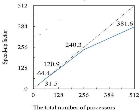
Fig. 10 The relationship between the total number of processors and the speed-up factor of the Earth Simulator.
