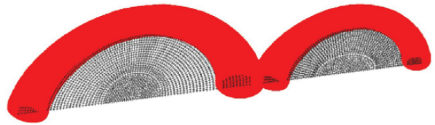
Fig. 2 Plastic zones along crack fronts.
