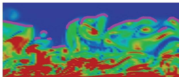
Fig. 1 A contour plot of the magnitude of vorticity near the wall of turbulent boundary layers. The contour curve (pink) defined by  $\omega = \omega_c = 0.7(U_\infty/\delta)$  captures well the T/NT interface of the TBL.
