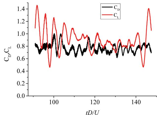
Fig. 5 The time histories of drag and lift coefficients.
