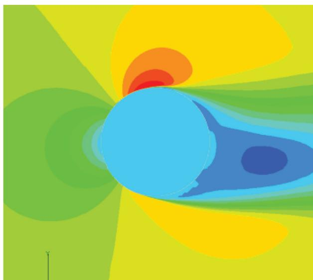
Fig. 6 The contours of time-averaged velocities.
