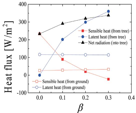
Fig. 4 Effect of the evaporation efficiency on the sensible, latent and radiative heat fluxes on the tree leaves and the ground surface.
