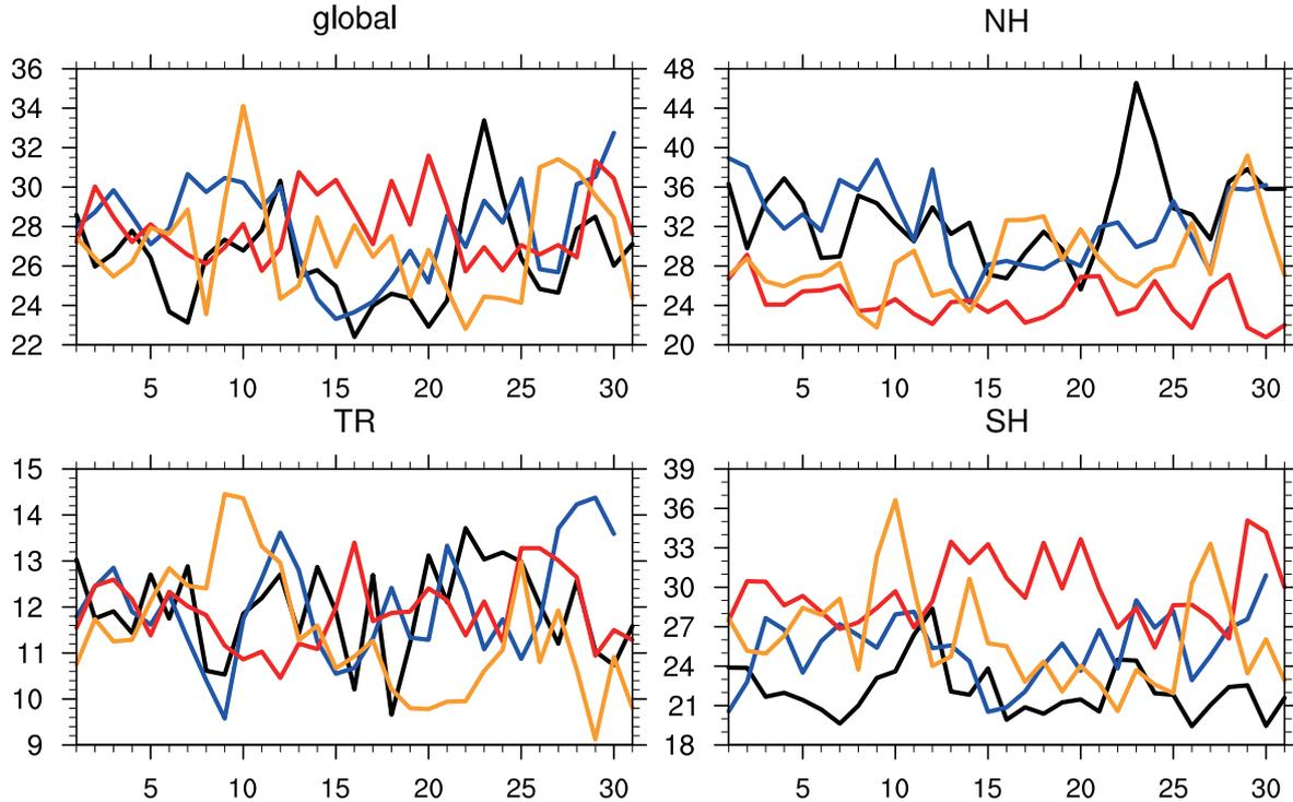
Fig. 1 The root-mean square error of the 48-h forecast of the geopotential height (gpm) at 500 hPa in the global domain (top left), in the Northern Hemisphere (top right), in the Tropics (bottom left) and in the Southern Hemisphere (bottom right) in the four-seasons experiment. The black, blue, red and orange curves represent the RMSE for January, April, July and October 2010, respectively. The horizontal axis indicates the initial dates.
