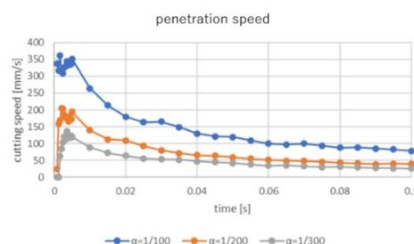
Fig. 3: Results of simulation by changing absorption parameter  $\alpha$
