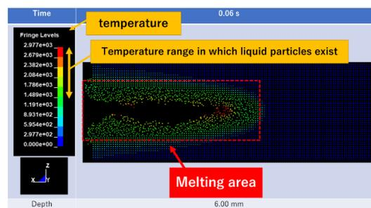
Fig. 4: Snapshot of melting simulation
