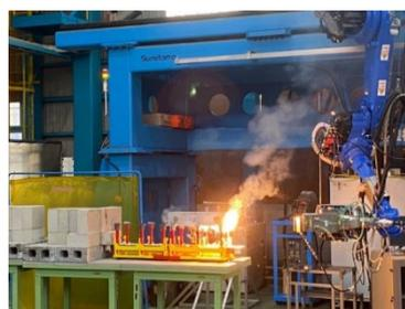
Fig. 1: High power laser induced concrete melting experiment
