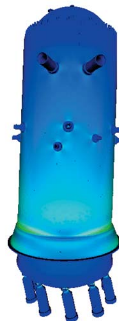
Fig. 10 Stress distribution and deformed shape of the ABWR model with 35 million DOF
