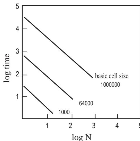
Fig. 1 Cpu time(second) vs size of parallel computing (number of nodes) for MD simulation of the 1000 to 1000000 atoms in the basic cell.
