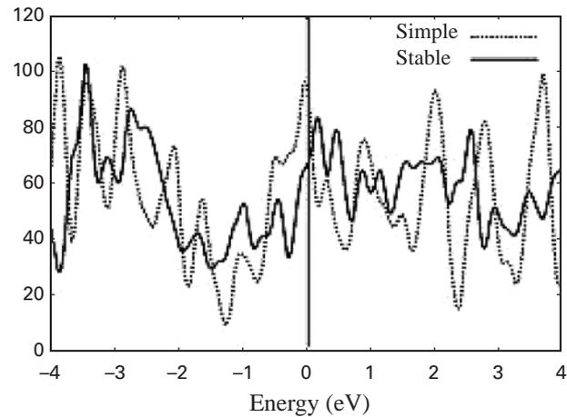
Fig. 3 Density of states of CNT-Ti contacts.
