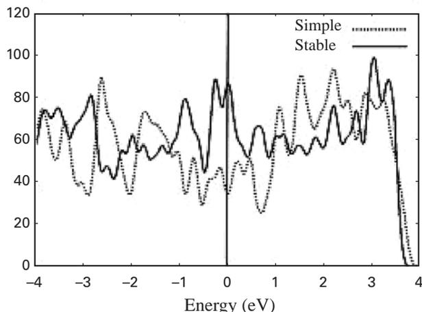
Fig. 5 Density of states of CNT-Mo contacts.
