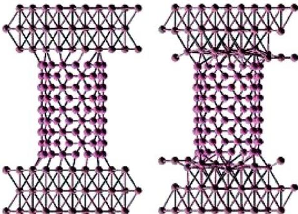
Fig. 2 Simple and stable atomic structures of CNT-Ti contacts.
