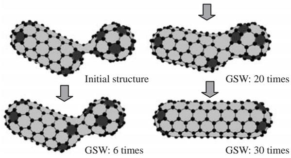
Fig. 8 Generation of capped CNT from two fullerenes.
