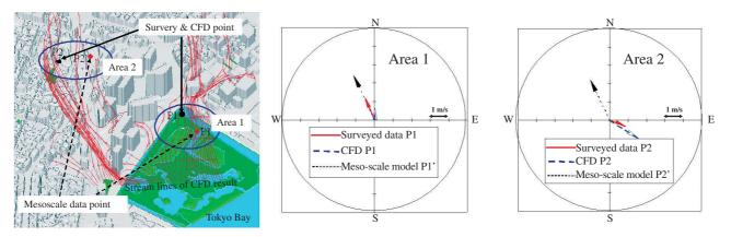
Fig. 4 Wind directions at 14:00: Surveyed result, CFD and mesoscale model. Middle figure: Area 1 (at the seaside). Right figure: Area 2 ( in the town).
