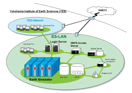
Fig. 3 Network Composition around the Earth Simulator
