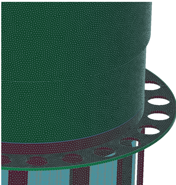
Fig. 1 The FE mesh around of a shroud inside of the BWR pressure vessel.
