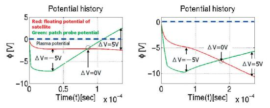
Fig. 4 Potential variation of single patch probe in the plasma environment without electron flux (left), and with electron flux (right).
