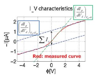
Fig. 6 Current-Voltage curve obtained for the double probe.
