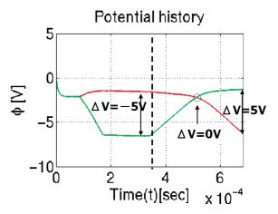
Fig. 5 Potential variation of double probe.
