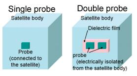
Fig. 2 Single- and double- Langmuir probe.
