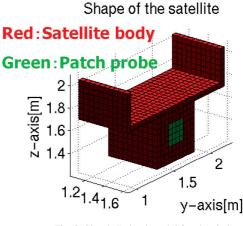
Fig. 3 Simple Reimei model for simulation.
