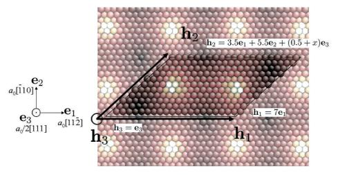
Fig. 2 The BCC iron supercell consisting of 231 atoms. The parameter x corresponds to the shear strain  $\gamma_{23}$ .
