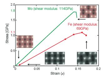
Fig. 3 Stress-driven instability of dislocation cores for BCC Mo and Fe: The shear modulus is derived from the inclination of the stress versus strain curve, and Peierls stress is determined from the maximum value of stress. The inset pictures show the positions of dislocation cores before and after the instability occurs.
