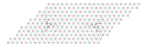
(a) Differential displacement map of threefold degenerate core structure
