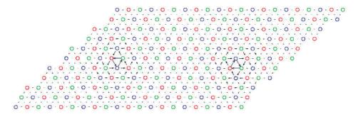
(b) Differential displacement map of symmetric non-degenerate core structure
