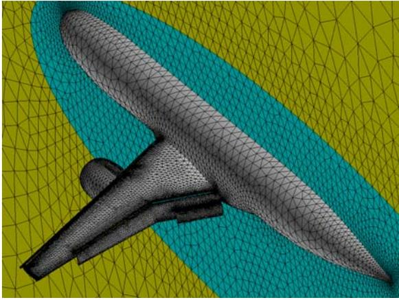
Fig. 3. Computational mesh around JAXA high-lift configuration model.
