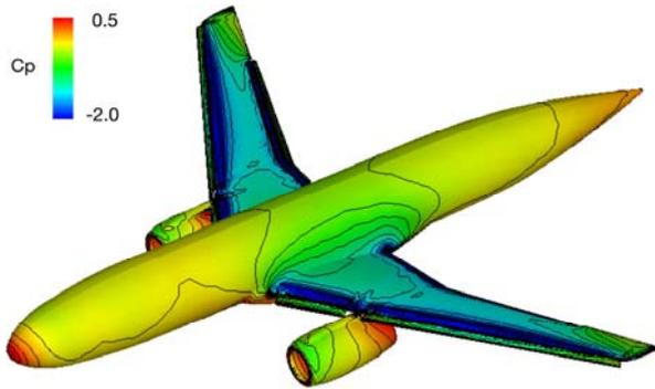
Fig. 4. Pressure contours on the surface of JAXA high-lift configuration model.
