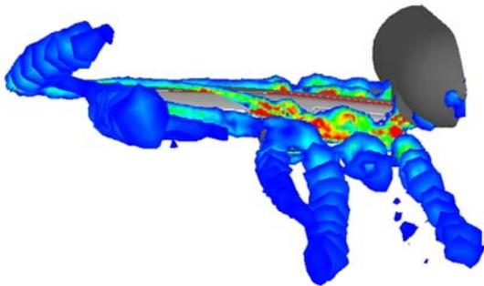
Fig. 6. Vorticity contours on several cross sections in the downstream region.
