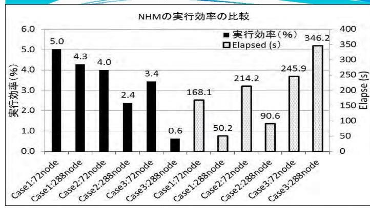
Case 1: To measure physical computation part in the main loop excluding initial files and file output.
