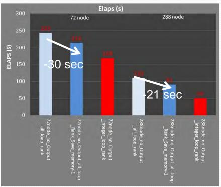
Light green: Output node and no Save Memory Deep green: Output node and Save Memory Red: Compute physical loop
