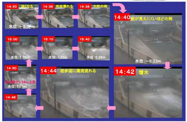
The water level increased 1.34m for 10 minutedue to unexpected rain. After this disaster, Kobe city has installed automatic early warning system for selected small rivers.
