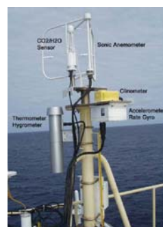
Fig. 2.7-1. Turbulent flux measurement system on the top deck of the foremast.
