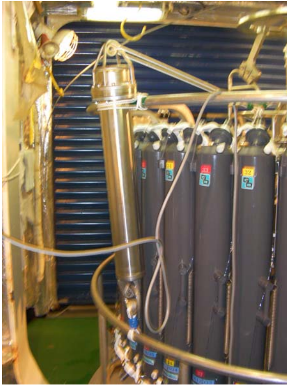
Figure 4.15-2. Acoustic release lashed to CTD frame for the response test of acoustic release in deep sea.
