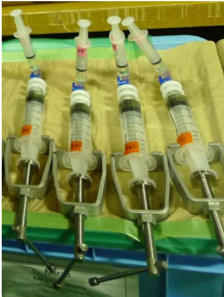
Fig. 4.14.2-1. System of squeezing pore water from sediment samples
