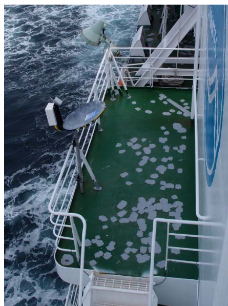
Figure 2.4-2: The micro rain radar, installed on the starboard side of the anti-rolling tank.
