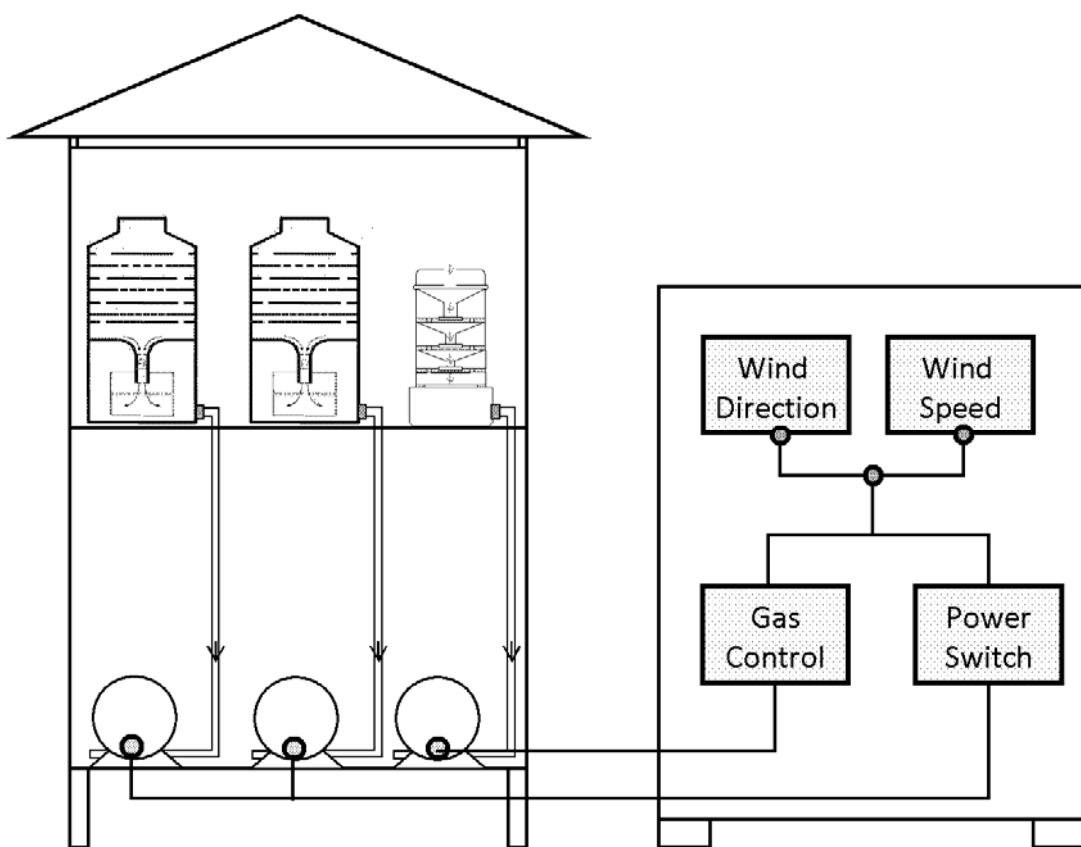
Figure 2.9-3: Schematic diagram of Cascade impactor sampling system
