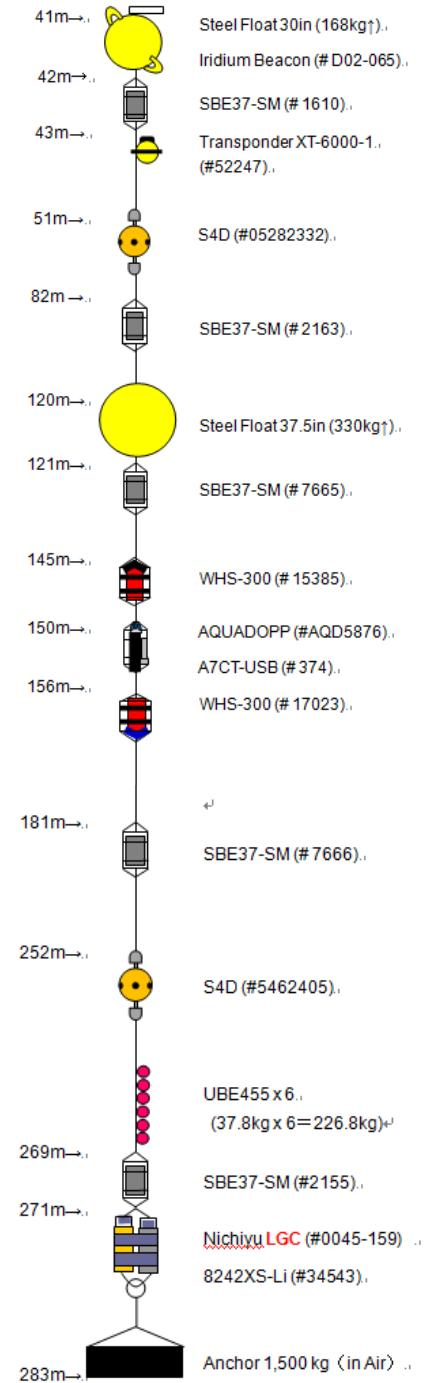
Figure 3.9-1: Diagrams of deployed moorings (BCW-15, BCE-15, and BCC-15).
