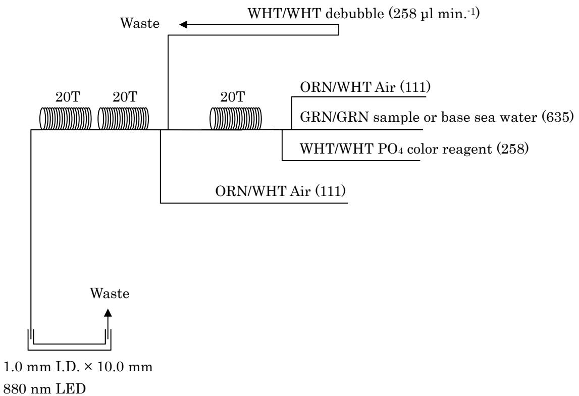
Figure 4.2-4 PO<sub>4</sub> (4ch.) Flow diagram.
