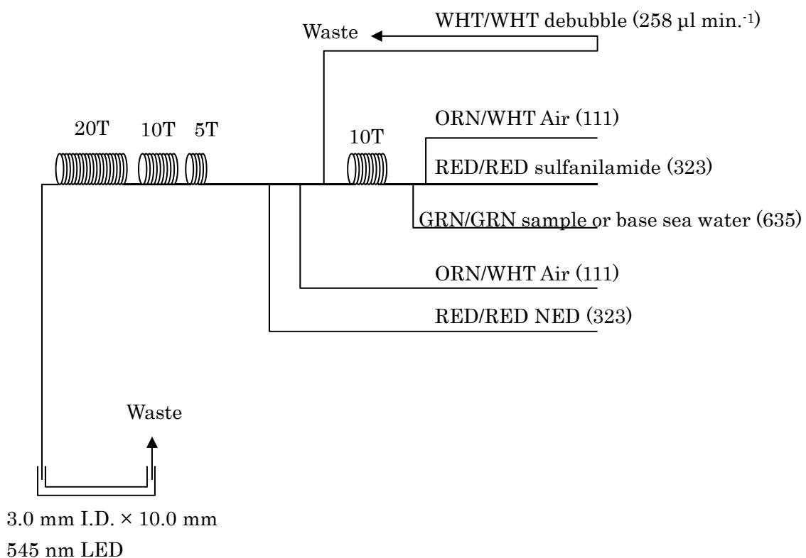
Figure 4.2-2 NO<sub>2</sub> (2ch.) Flow diagram.
