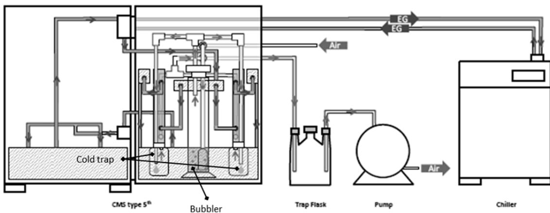
Figure 2.9-2: Schematic diagram of CMS type 5<sup>th</sup> system
