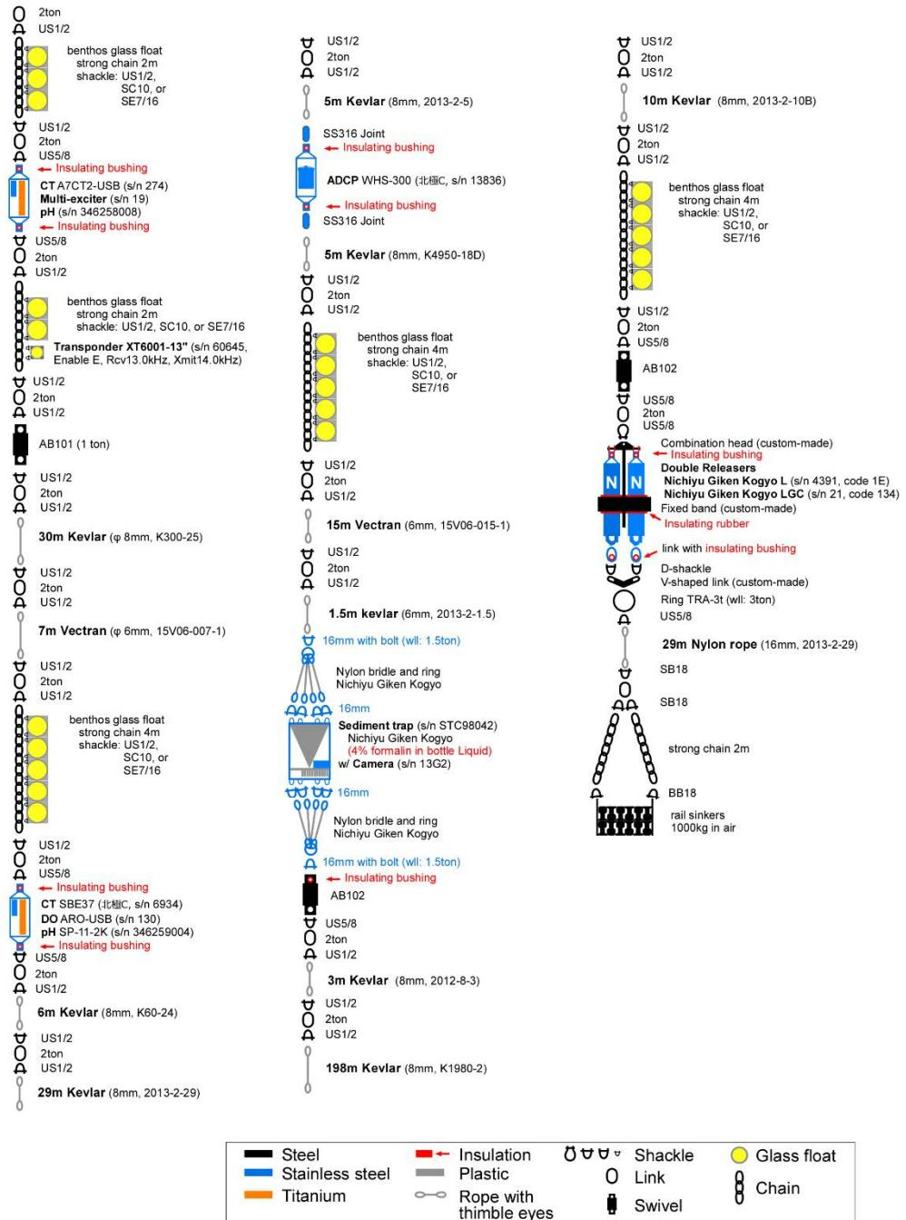
Fig. 4.21-5: The design of sediment trap mooring NHC15t.
