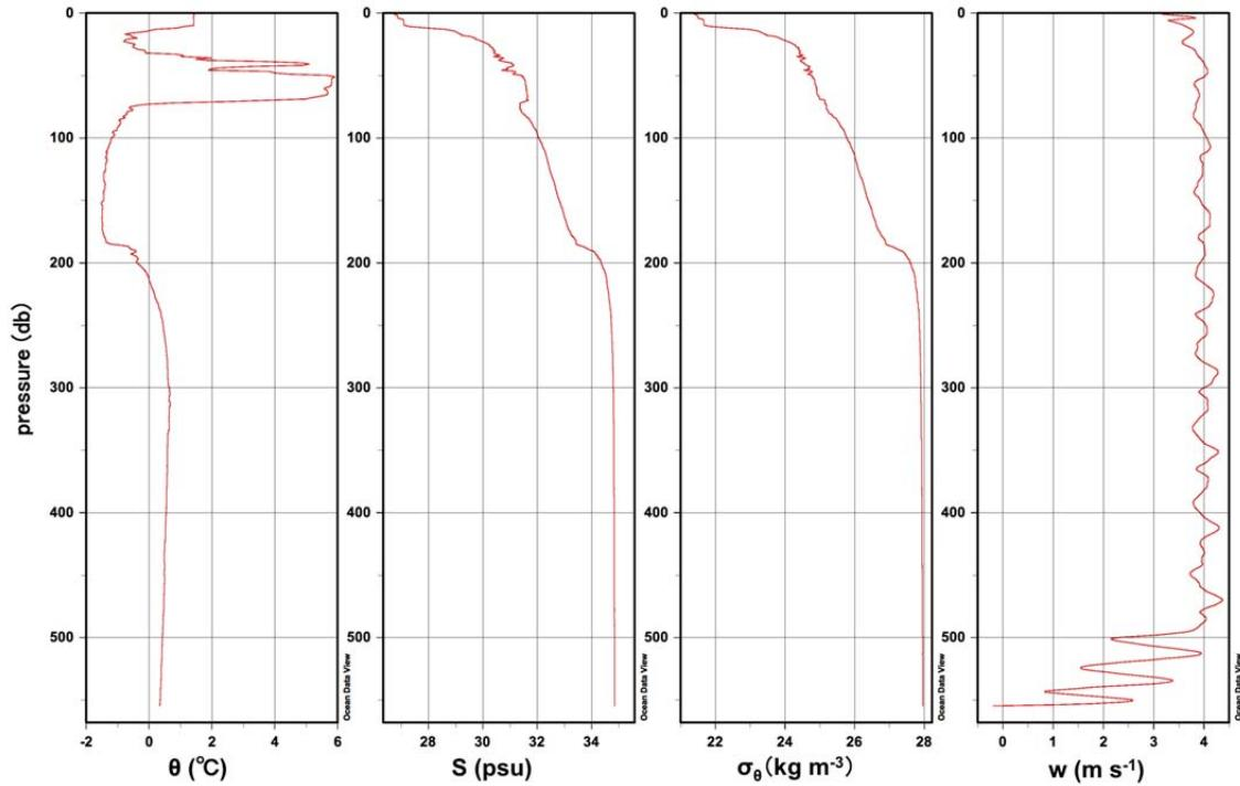
Figure 3.3-2: Typical profiles from U-CTD observation of (a) potential temperature  $\theta$  (deg-C), (b) salinity  $S$  (practical salinity unit), (c) potential density  $\sigma_{\theta}$  ( $\text{kg m}^{-3}$ ), and (d) descending rate  $w$  ( $\text{m s}^{-1}$ ) at a station of u003c01, positioned off the Barrow Canyon.
