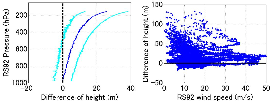
Figure 2.1-5: Mean difference of altitude between RS92-SGPD and RS41-SGP. Differences were calculated at the same observation time. Blue and cyan lines in the left panels denote mean difference and standard deviation.
