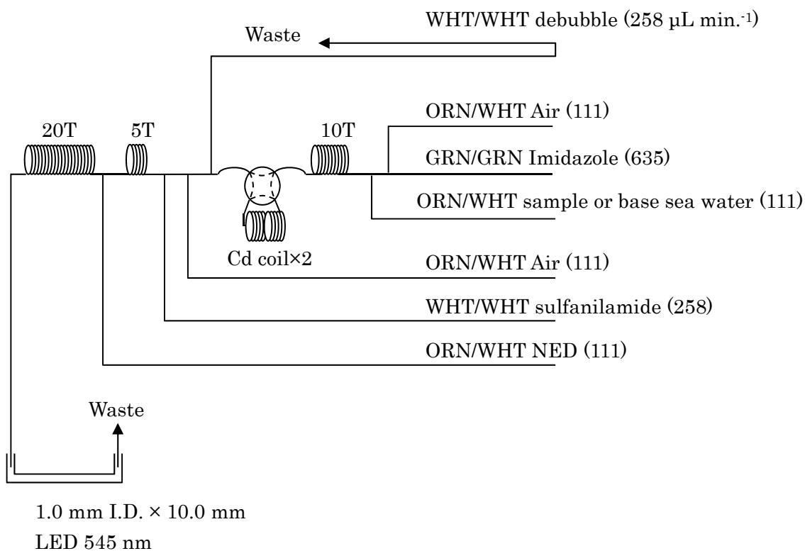
Figure 4.2-1  $\text{NO}_3 + \text{NO}_2$  (1ch.) Flow diagram.
