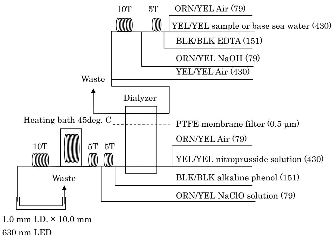
Figure 4.2-5 NH<sub>4</sub> (5ch.) Flow diagram.
