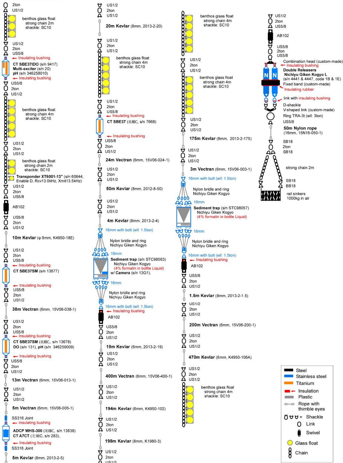
Fig. 4.21-3: The design of sediment trap mooring NBC15t.
