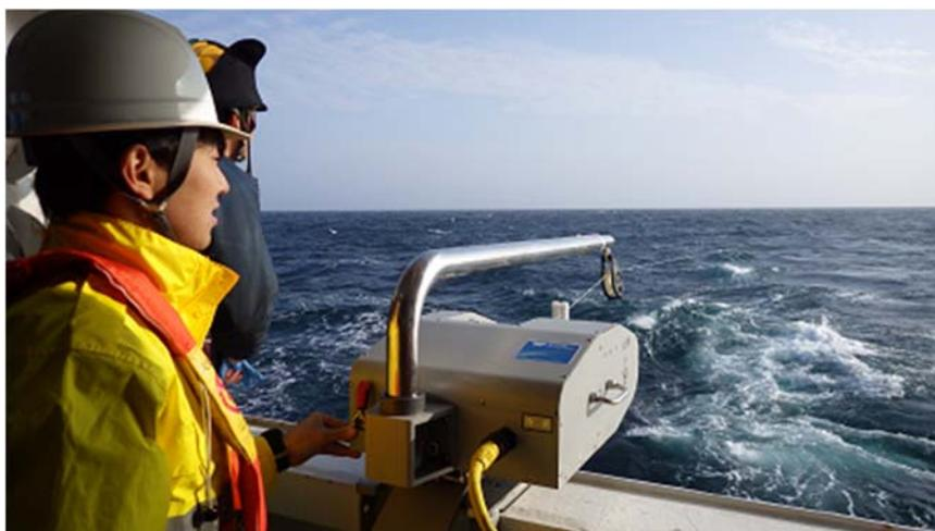
Figure 3.2.2-1: UCTD system installed and operated on R/V Mirai.
