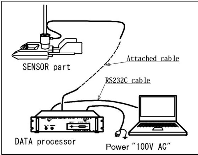
Figure 2.5-1: Schematic view of spray particle counter (SPC).
