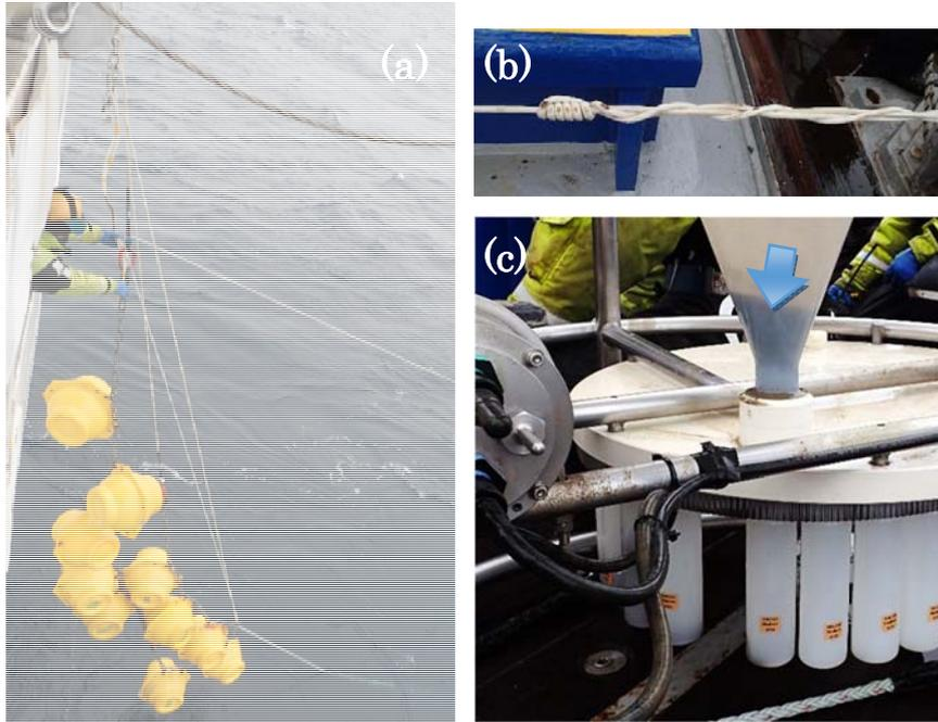
Figure 4.16.1-4: (a), (b) tangled mooring line of NBC15t, and (c) NBC15t shallow trap on deck. The blue arrow shows particle clogging at the bottom of trap cone.
