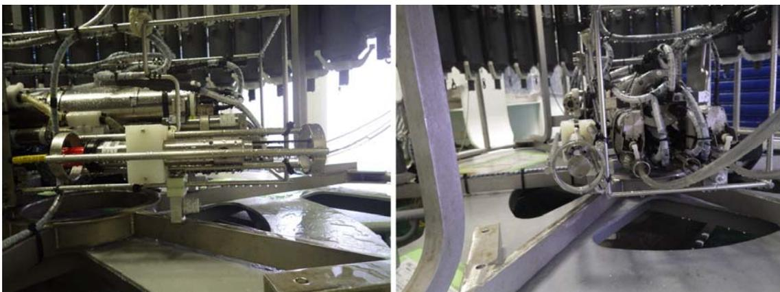
Fig. 3.10.1. Photos of the velocimeter attached to the CTD frame.
