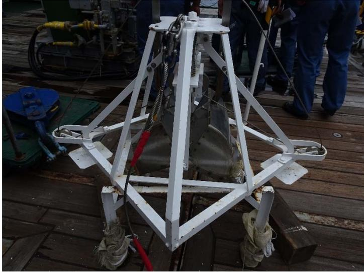
Figure 4-17-1. Picture of the Smith and McIntyre grab sampler.
