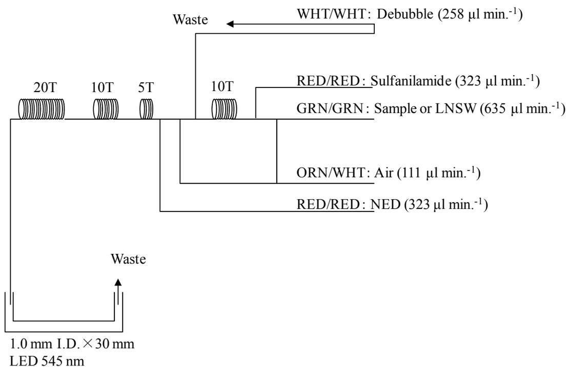
Figure 4.2-2 NO<sub>2</sub> (2ch.) Flow diagram.
