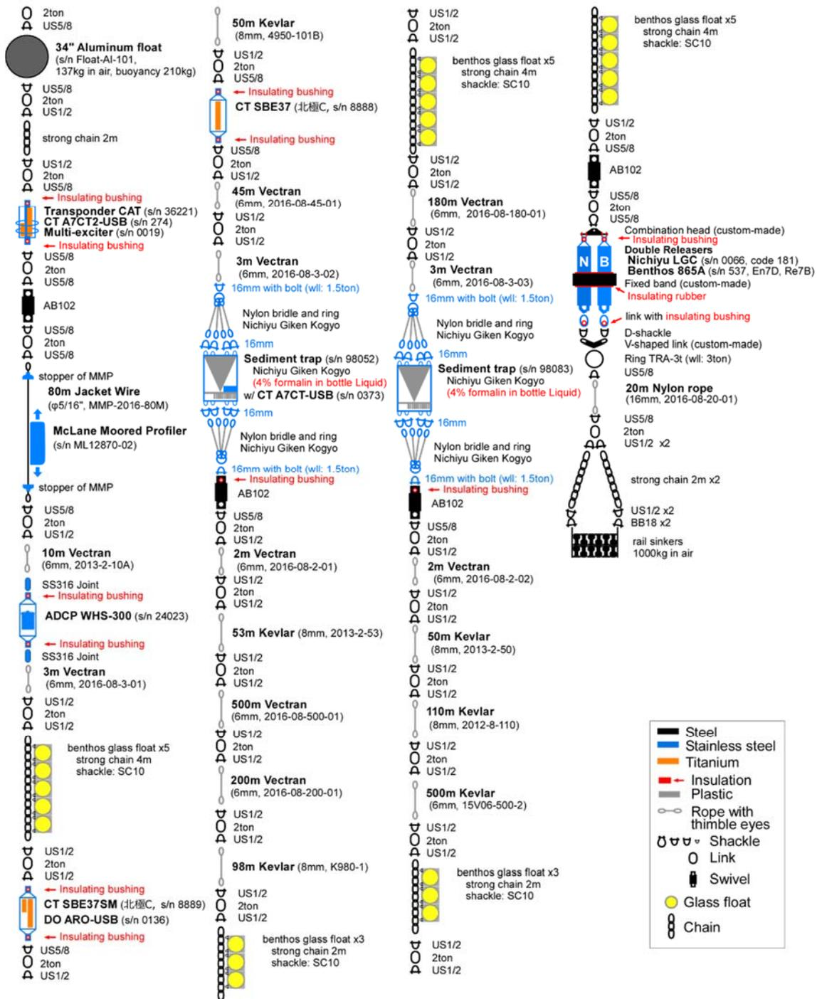
Figure 4.16.1-8. The design of deployed sediment trap mooring NBC16t.
