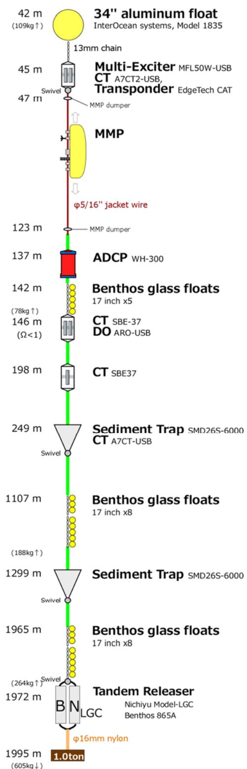
Figure 4.16.1-6. The outlined design of sediment trap mooring for deployment in Canada Basin.
