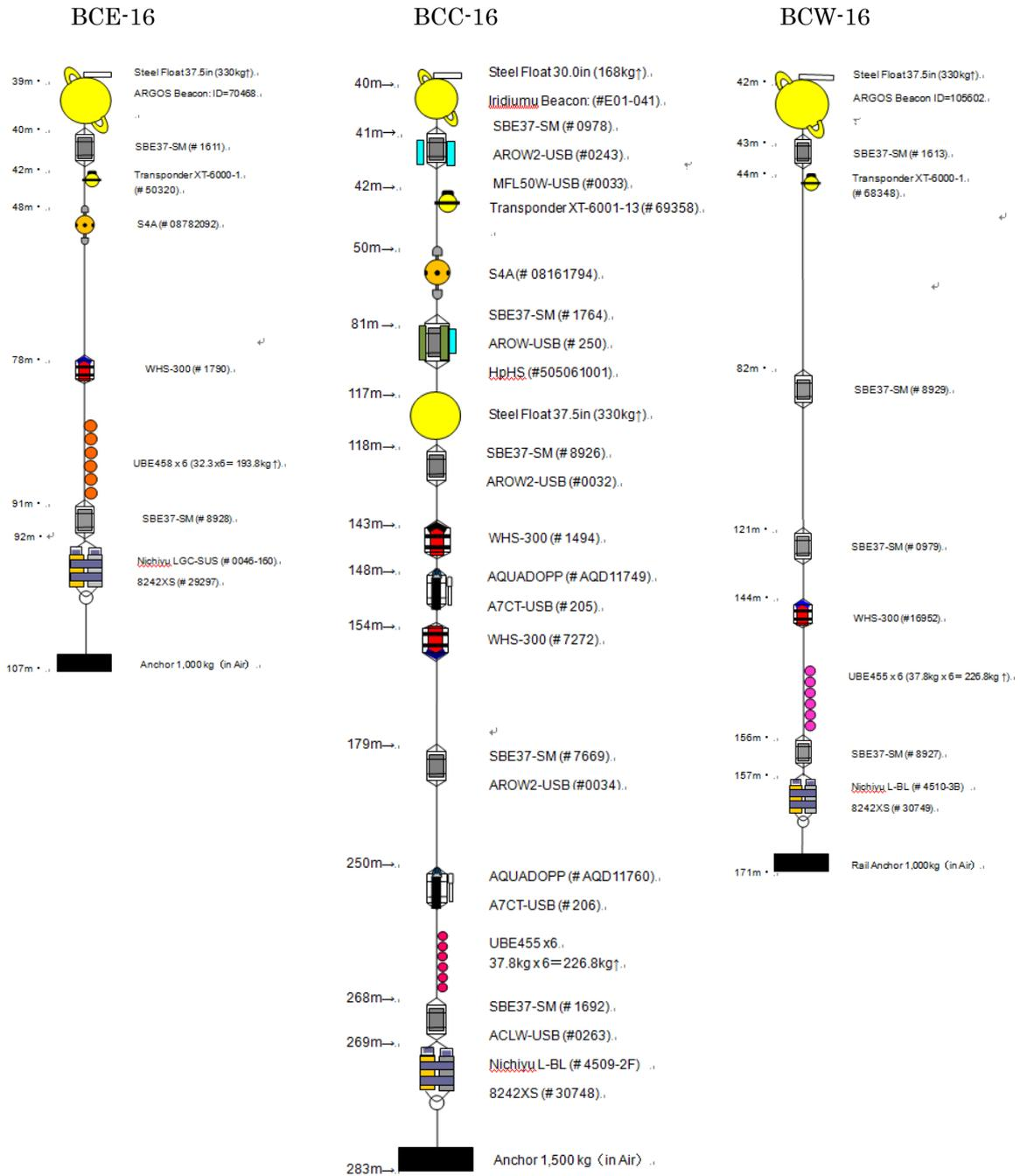
Figure 3.8-1: Mooring diagram of Deployment moorings (BCE-16, BCC-16, BCW-16)
