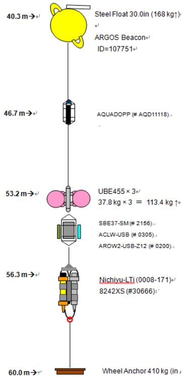
Figure 3.8-2: Mooring diagram of Deployment moorings (SCH-16)
