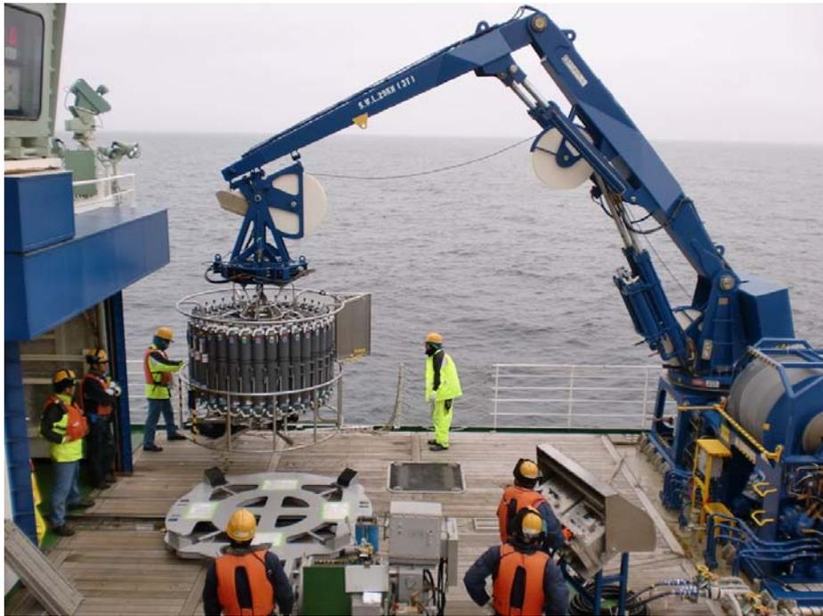
Photo 1.2-2. Oceanographic observation using Conductivity-Temperature-Depth (CTD) sensors and water sampling bottles.
