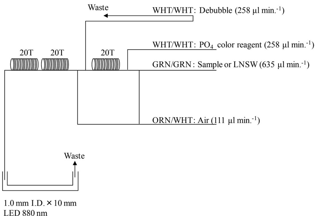
Figure 4.2-4 PO<sub>4</sub> (4ch.) Flow diagram.
