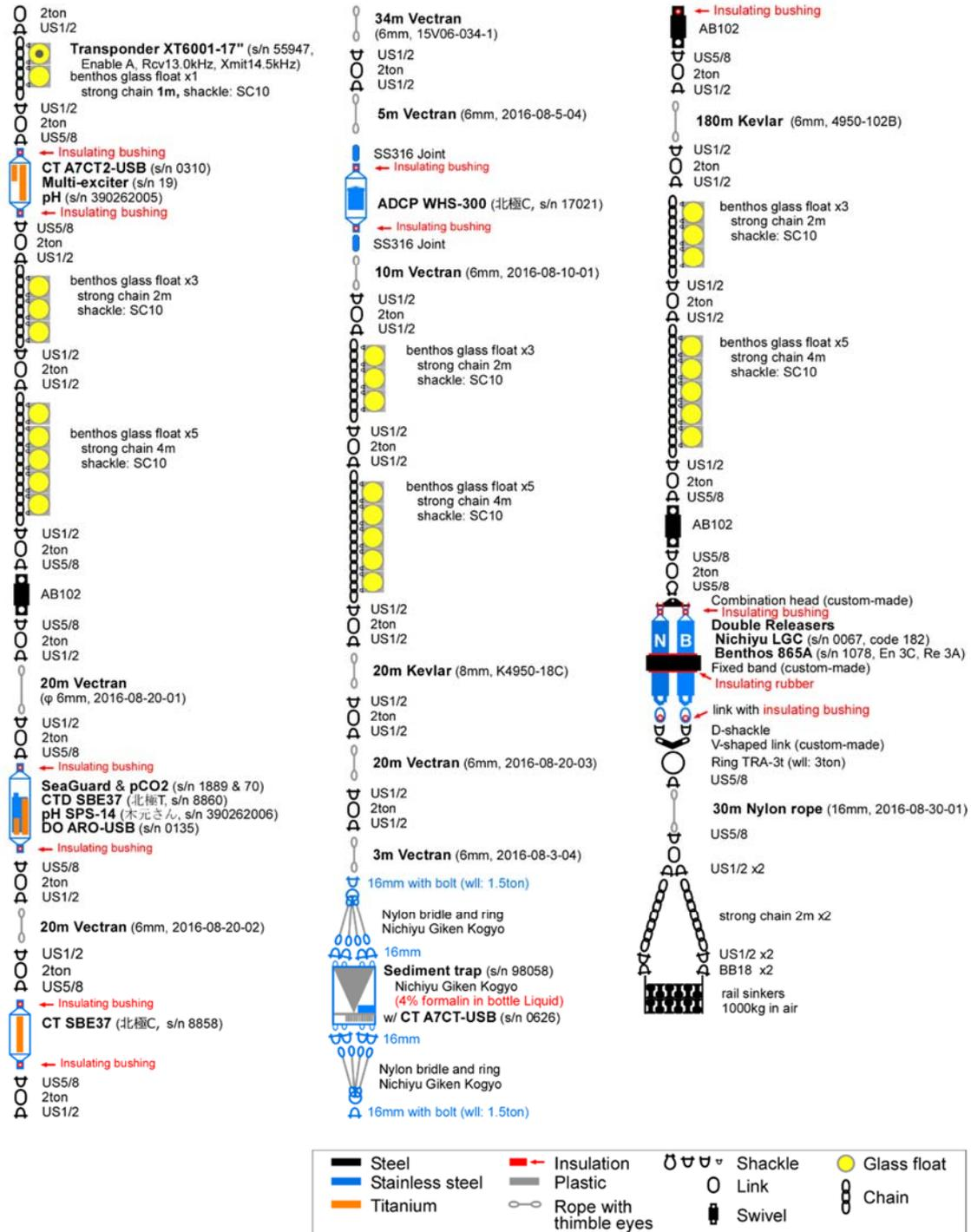
Figure 4.16.1-7. The design of deployed sediment trap mooring NHC16t.
