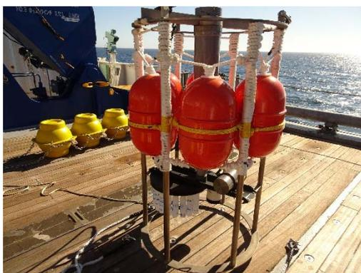
Figure 4.16-2-1. Picture of the sediment trap.
