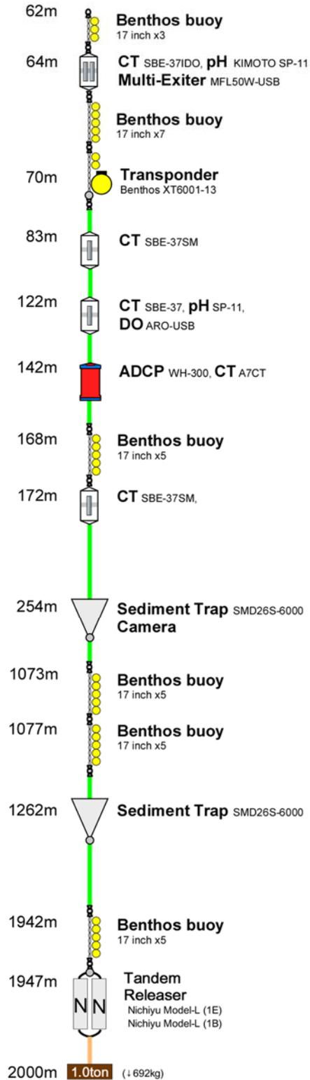
Figure 4.16.1-3: The outlined design of sediment trap mooring for recovery.
