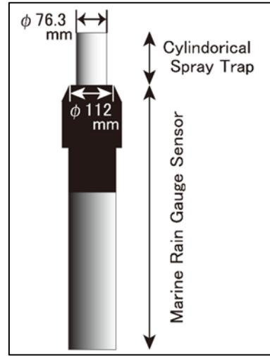
Figure 2.5-2: Schematic view of marine rain gauge type spray gauge (MRS).
