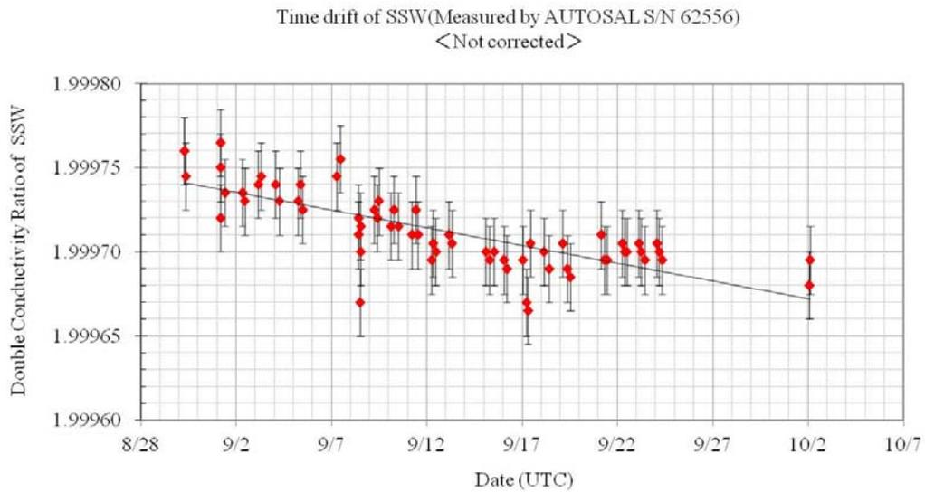
Figure 3.5-1 History of double conductivity ratio for the Standard Seawater batch P159 in the salinometer S/N 62556 (before correction)
