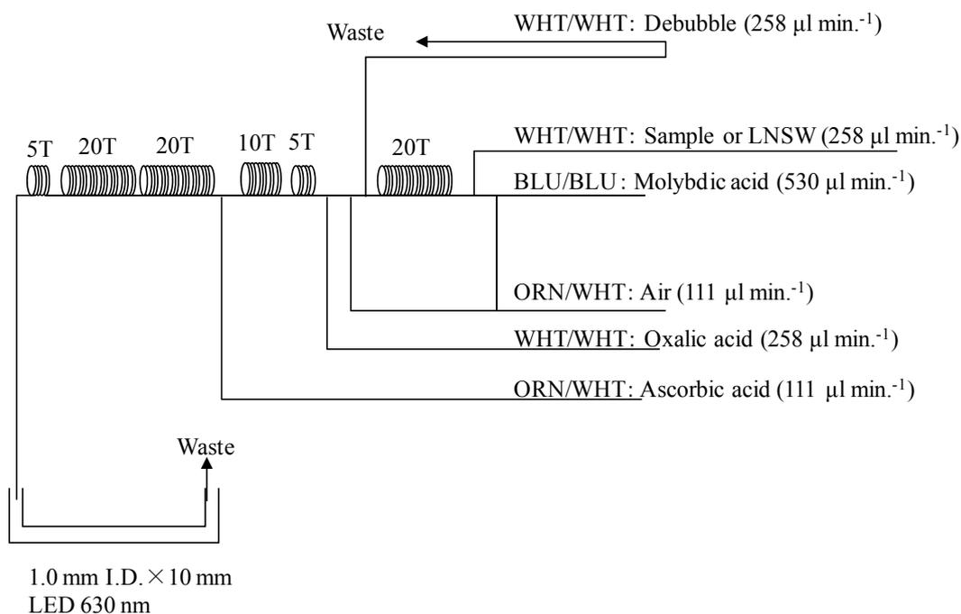
Figure 4.2-3 SiO<sub>2</sub> (3ch.) Flow diagram.
