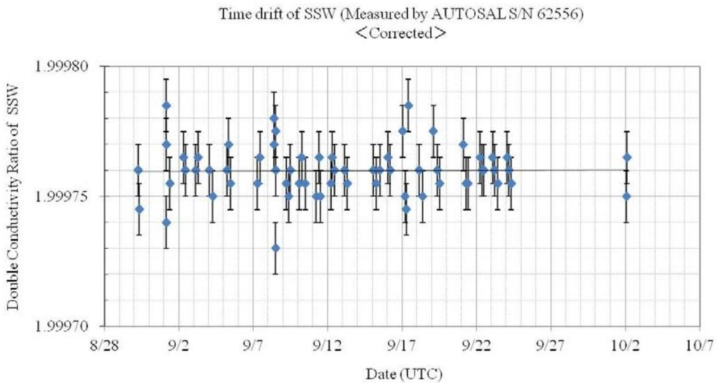
Figure 3.5-2 History of double conductivity ratio for the Standard Seawater batch P159 in the salinometer S/N 62556 (after correction)
