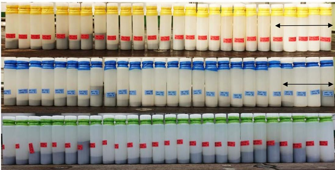
Figure 4.16-5: Recovered sediment trap bottles. Upper bottle line with yellow neck and middle line with blue neck is from the upper and lower sediment trap of NBC16t, respectively. Lower bottle line with pale green neck is from NHC16t. Left side is older (autumn 2016) and right end is this summer (Sep. 2, 2017). Arrows show the period for the clogging of trap cone.
