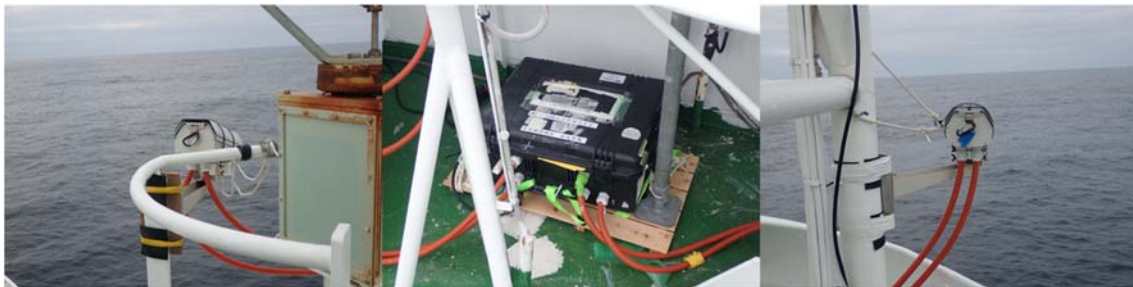
Figure 3.8-1. Stereo Camera System on the compass deck (Left: Left camera, Center: housing box, Right: Right camera).
