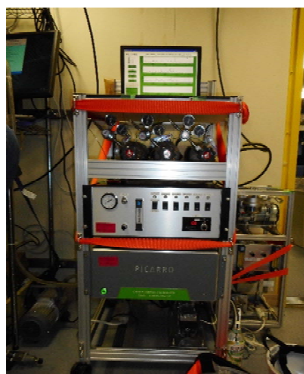
Photo 2.6-1. Continuous measurement system of the atmospheric CO 2 , CH 4 , and CO based on a cavity ring-down spectrometer (CRDS) used during MR20-05C cruise.
