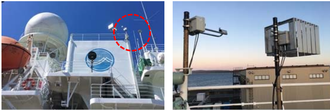
Figure 2.5.4-1. Onboard LPM sensors. (Left) The location of the sensors, as designated by the red broken circle. (Right) The sensors. Right one (aft one) equipped wind protection element to reduce the effect of the wind, while left one (fore one) did not.
