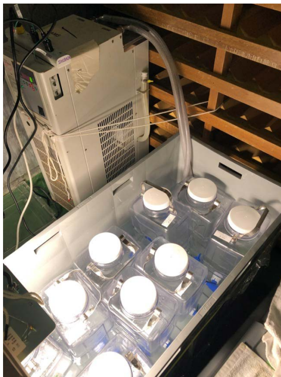
Photo 4.19.2: Temperature and light controlled incubation experiment system
