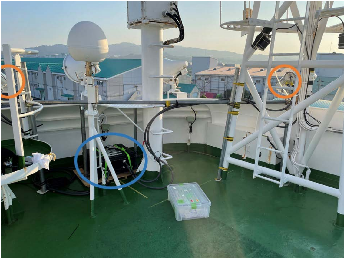
Figure 3.8-1: Installed stereo camera system. Cameras are indicated with orange circles, and the logger box is indicated with blue circle.
