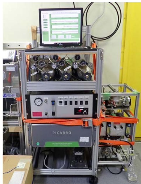
Photo 2.9-1: Continuous measurement system of the atmospheric CO 2 , CH 4 , and CO based on a cavity ring-down spectrometer (CRDS) used during MR21-05C cruise.
