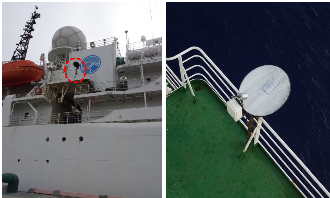
Fig. 2.3-1: Onboard MRR sensor. (Left) The location of the sensors, as designated by the red broken circle. (Right) The antenna unit.
