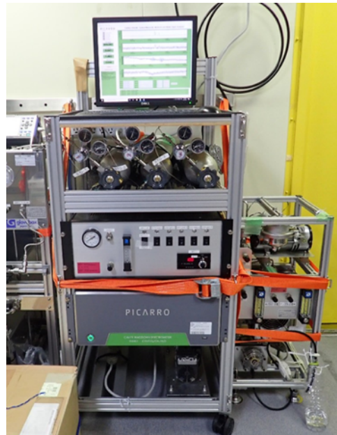
Photo 3.14-1. Continuous measurement system of the atmospheric CO 2 , CH 4 , and CO based on a cavity ring-down spectrometer (CRDS) used during MR23-06C cruise.
