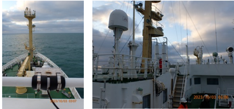
Figure 3.6-3 Network cameras installed on the compass deck.
