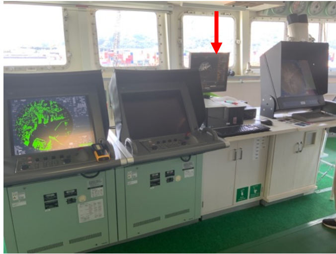
Figure 3.6-2 X-band wave analysis system installed in the bridge.
