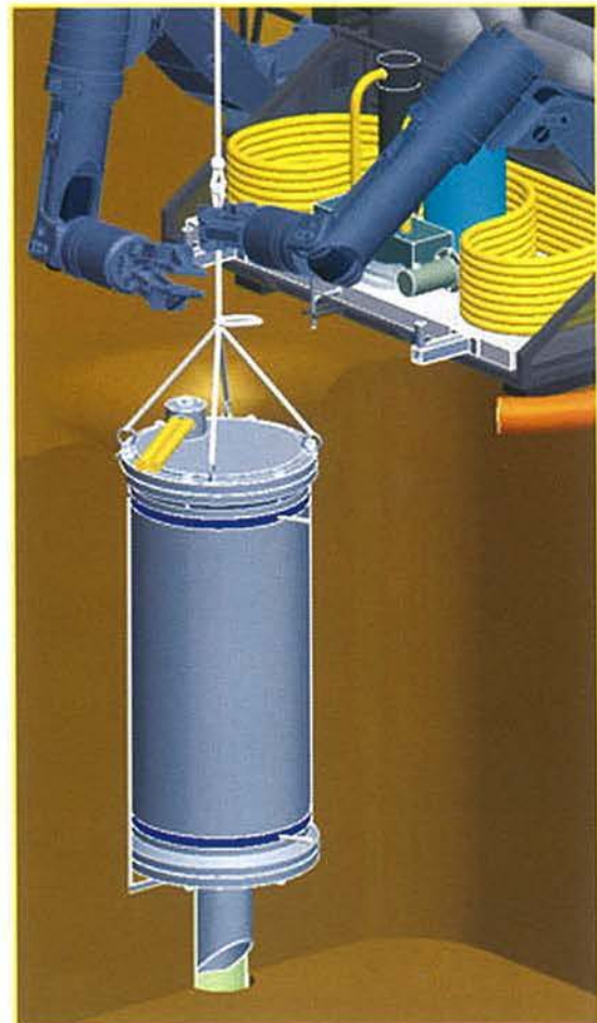
Fig. 6 Buried Observatory (Ground Motion Sensing System) The ground motion sensing system is buried in a sediment layer to reduce the background noise level from seafloor environment.
