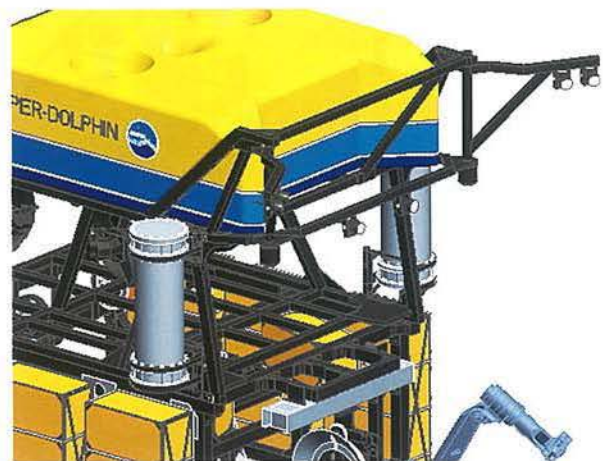
Fig. 10 Variable Buoyancy Control System The VBCS is a system able to adjust the buoyancy of the ROV by pouring or draining seawater to the pressure resist water tank. It is equipped a pair of 50 L volume pressure resisted water tanks to compensate the 1 kN of buoyancy additionally in water to maintain the mobility of the ROV in cable laying operation.
