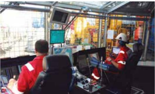
The driller's house ("Dog House") is where all drilling and downhole operations are controlled and monitored. A modern digital system assists the drillers in manipulating all tools and equipment on the drill floor, and monitors downhole conditions in realtime. The BOP control system are also controlled and monitored from here.
