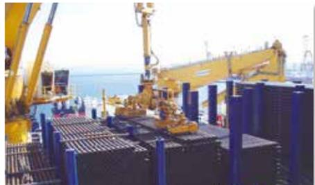
Pipe racks (fore & aft) store drill pipes (each joint ca. 9.5 m) and casing pipes. 10,000 m of drill pipes can be stored. Other tools and equipments for downhole can be stored here as well.
