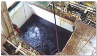
A 22 m x 12 m rectangular opening located amidship. All drilling, coring, and riser operations use this opening to the sea floor.
