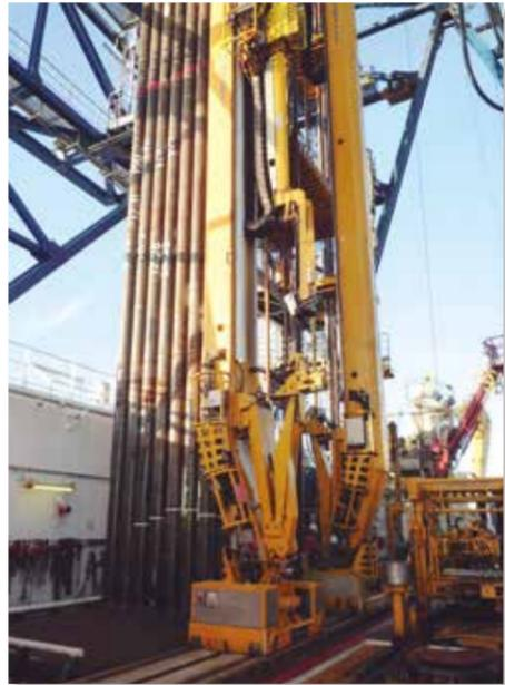
The pipe racker moves pipe stands (3-4 connected joints of drill pipe) from the standby vertical pipe racks to the well center in the middle of the drill floor. There are 23-armed pipe rackers on the rig floor, remotely controlled from the driller's house.
