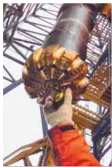
Poly-crystalline diamond compact (PDC) core bit drills and trims core samples. The coring systems are designed for differing sediment or rock hardness, and the PDC bits are also specifically designed according to the formation being drilled.
