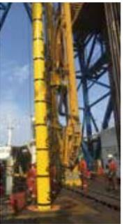
Special large-diameter pipe placed inside a borehole, to protect the borehole from collapsing. Casing pipe allows a borehole to be re-entered with special logging tools, coring tools, deepen the borehole, or place special sensors to measure and record the characteristics of the deep sediment/rock formations.
