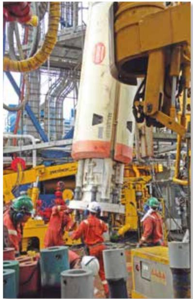
Special larger diameter, bouyant pipe to connect the mud circulation system to the seafloor, making the circulation a closed system. Drill pipes and tools pass through the center, and drilling mud and cuttings return to *Chikyu* for recycling.
