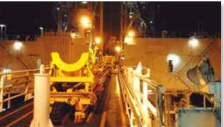
The riser pipe transfer system (RTS) helps move riser pipes to and from the rig floor, and it can be used to move other heavy objects to the rigfloor as well.
