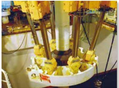
Special hydraulic pistons to secure the riser pipe to *Chikyu*, which also can apply slack or tension on the riser pipe, as needed. They help neutralize some of the heave from *Chikyu's* motion in the ocean while drilling under DPS.
