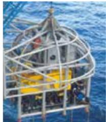
The *Chikyu* has an ROV able to operate ca. 3,000 m below sea level. The ROV is equipped with B/W and color TV cameras, 2 manipulator arms, and can use other tools as needed.
