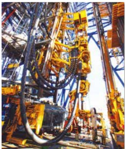
Top Drive System (HPS: Hydralift Power Swivel) is a special motor inside the derrick that raises, lowers, and rotates the drill pipe, and also allows drilling mud to be pumped, downhole. The HPS can hold 10,000 m of drill pipes and tools.
