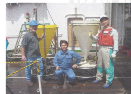
Working on the deck of the RV Mirai, Dr. Makio Honda with colleague, and myself are preparing time-series sediment traps from JAMSTEC and the Woods Hole Oceanographic Institution for deployment in the North Pacific.
