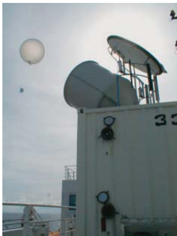
Fig. 1 Launch the radiosonde from container.
