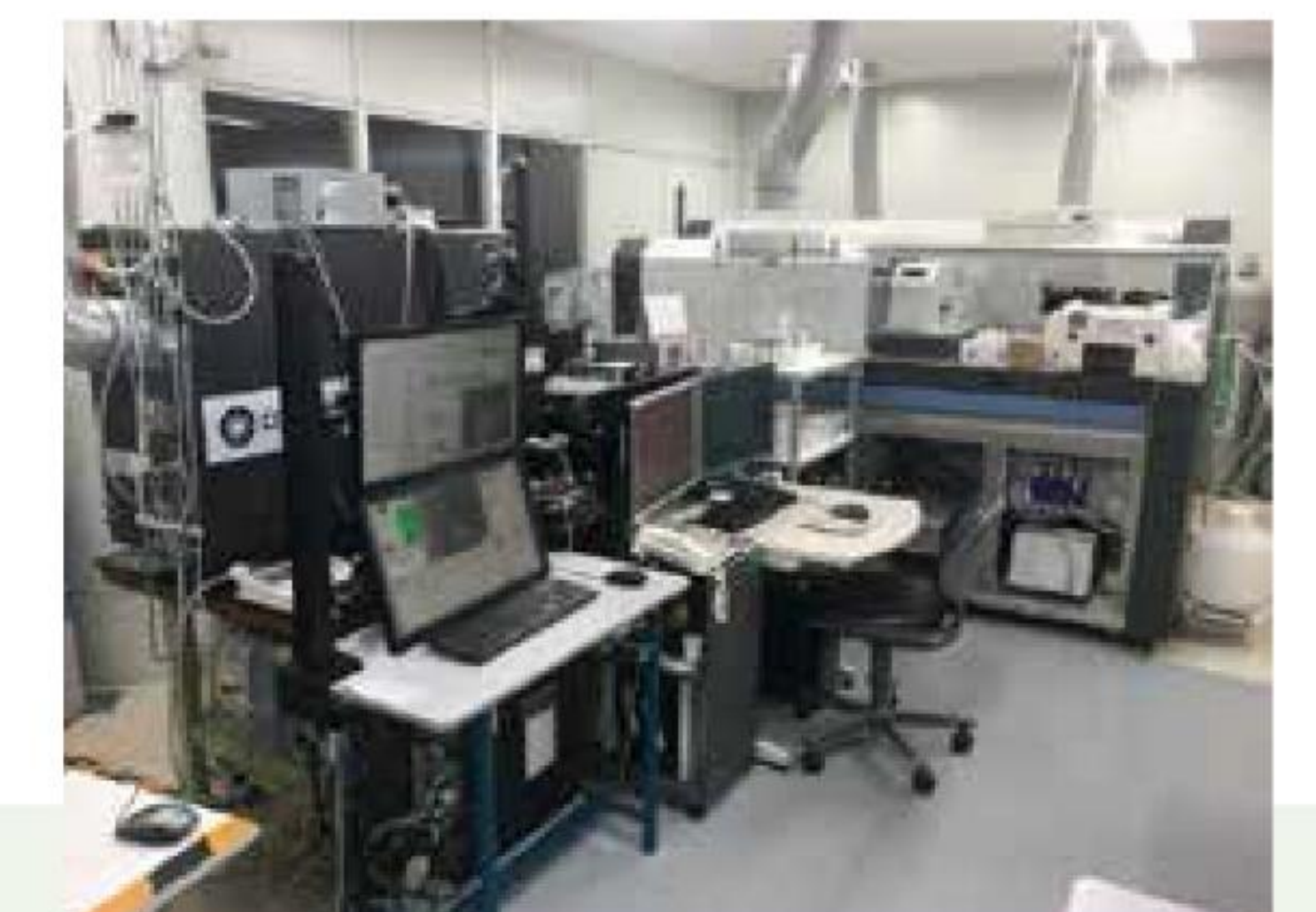
Laser ablation inductively coupled plasma mass spectrometer (LA-ICP-MS) uses to determine rock compositions.
