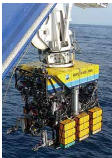
Fig 2. An example of using an ROV for sampling
