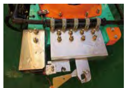
Fig.8 Disconnecter after use (Left: electrolytic method, Right: nylon line thermofusion method)
