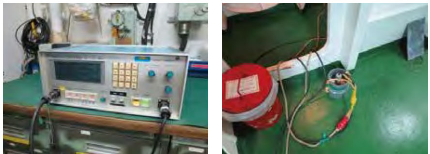
Fig.12 Transducer control unit (left) and transmitting unit (right)
