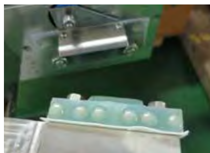
Fig.8 Disconnecter after use (Left: electrolytic method, Right: nylon line thermofusion method)
