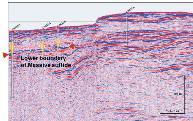
Fig. 4 Detailed cross section of ZVCS (source: Delta sparker). Drilling core information courtesy of JAMSTEC.
