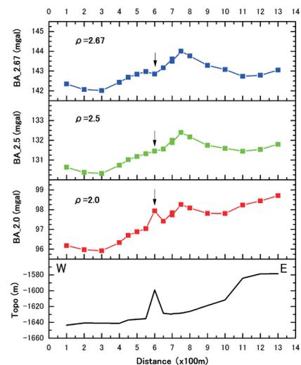
**Fig. 2** Simple Bouguer gravity anomaly profiles of three different cases of Bouguer collection densities, and topography (the bottom)
