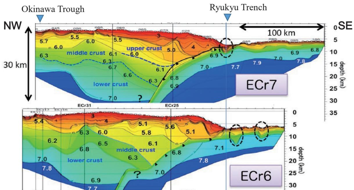
**Fig.1** P-wave velocity models in and around the Ryukyu Trench.
