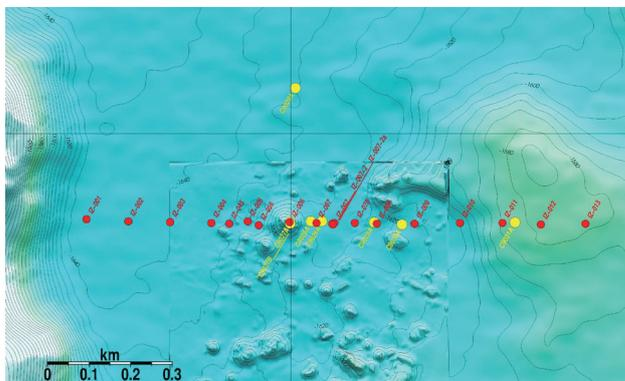
**Fig. 1** locations of the gravity measurement sites (red circles) and drilled sites by D/V Chikyu (yellow circles)
