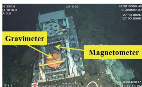
**Photo 1** Appearance of the simultaneous survey using the towing system of J-MARES
