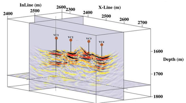
Fig. 2 Three dimensional sub-seafloor structure of VCS (source: GI gun).
