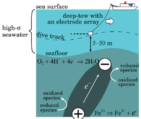
**Fig.1** Schematic figure of the chemical reaction of sub-seafloor related to the self-potential anomaly.
