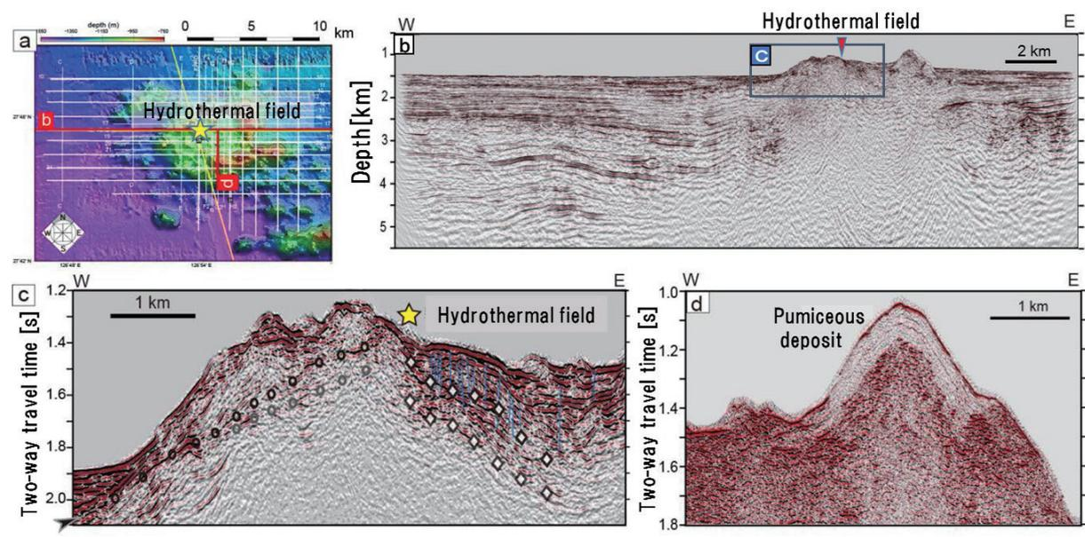
**Fig.1** Results of the seismic reflection survey around the Iheya North Knoll hydrothermal field.
