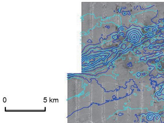
**Fig.2.** Backscatter strength with bathymetric contours
