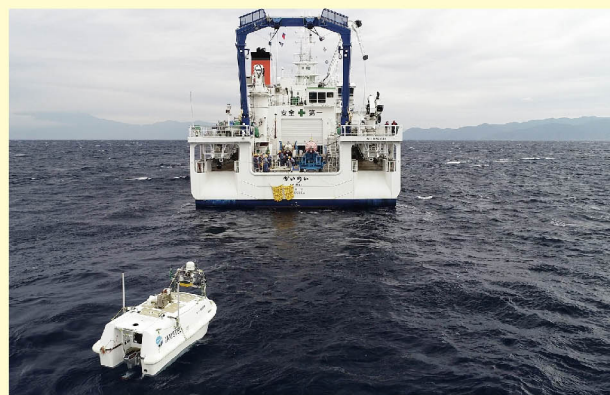
Sea trial of acoustic communication among the AUVs, the ASV, and the mother ship
