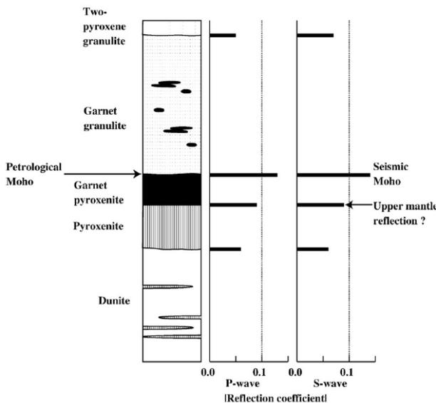
Figure 5. Schematic illustration for the lowermost crust and upper mantle of the Kohistan arc section and absolute values of the maximum reflection coefficients for P- and S-waves at each lithological boundary. From Kono et al. (2009)
