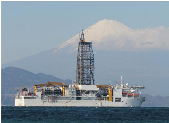
*Fig. 1. The riser-drilling platform D/V Chikyu.*
