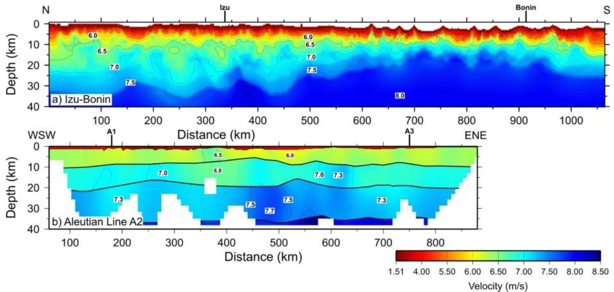
**Fig. 3.** (Top) Combined seismic velocity models along the modern volcanic line of the Izu and Bonin arcs (Kodaira *et al.* 2007b). Velocities are displayed with the same scale as Fig. 2. Vertical exaggeration is 4:1. (Bottom) The along-strike P-wave velocity structure of the Aleutian island arc (Shillington *et al.*, 2004).
