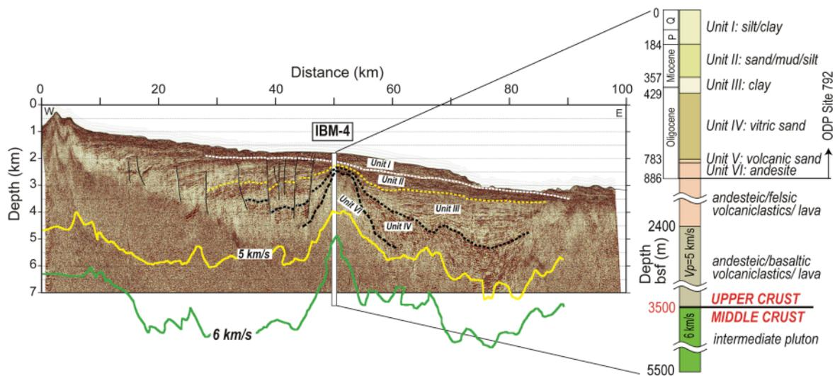
Fig. 1. Lithological interpretation of the seismic image along the IBM-4-EW5 section based on the results of ODP792 (Taylor et al., 1992). Iso-Vp contours of 5 km/s and 6 km/s obtained by wide-angle OBS data are also shown.
