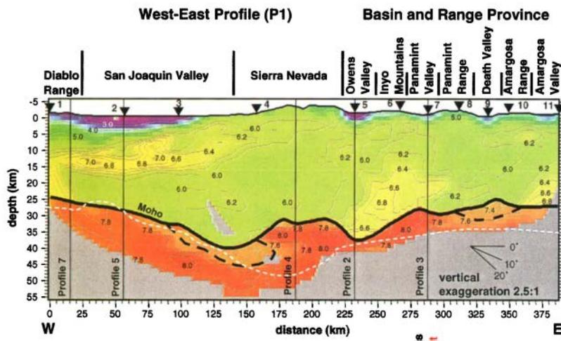
Fig. 9. Low seismic velocities ( $V_p=6.0\pm 0.2$  km/s) through most of the Sierran crust (Fliedner et al., 2000).
