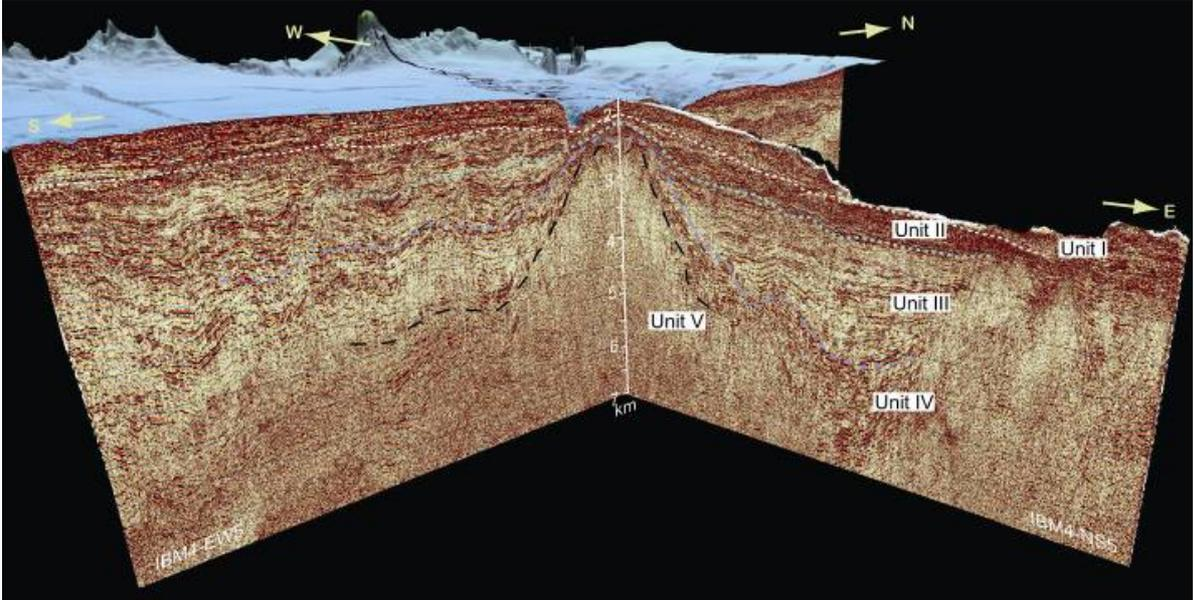
**Fig. 5.** 3D view of the seismic reflection sections crossing the IBM-4 Site. A conical basement high, which is likely to be composed of lavas and volcanoclastics, is well documented, suggesting the presence of an Eocene volcanic body beneath the IBM-4 Site.
