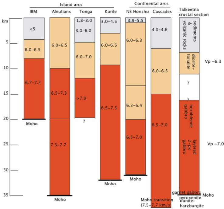
Figure 1. Seismic velocity profiles of various modern island arcs and continental arcs compared to the
