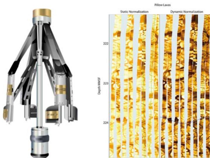
Figure 1. Left: Formation MicroImager (FMI), an electric microimaging wireline tool. Right: Formation MicroScanner (FMS) image from Hole 1347A, IODP Expedition 324, Shaysky Rise. Fractured pillows and dip direction of lava flow plane are well imaged.
