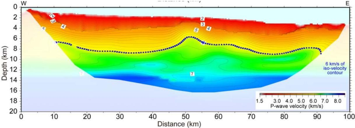
**Fig. 6** Seismic velocity image of the E-W profile at the proposed site.
