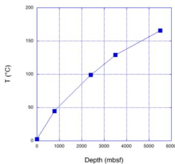
Fig. 2. One possible temperature estimate, assuming that thermal conductivity between 0-783 m, 783-2400 m, 2400-3500m, and 3500-5500m are 1.012, 1.610, 2 and 3, respectively.
