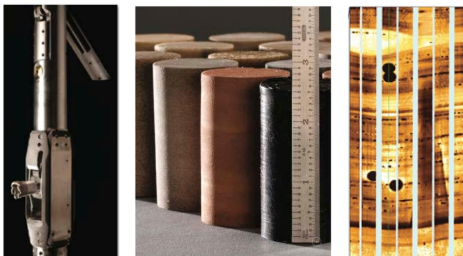
Figure 2. Left: Sidewall coring tool (XL-Rocks). Center: Samples taken by XL-Rock. Right: FMI images after sidewall samples were taken. Figures are taken from [http://www.slb.com/services/characterization/wireline\\_open\\_hole/rotary\\_sidewall\\_coring/xl\\_rock.aspx](http://www.slb.com/services/characterization/wireline_open_hole/rotary_sidewall_coring/xl_rock.aspx)
