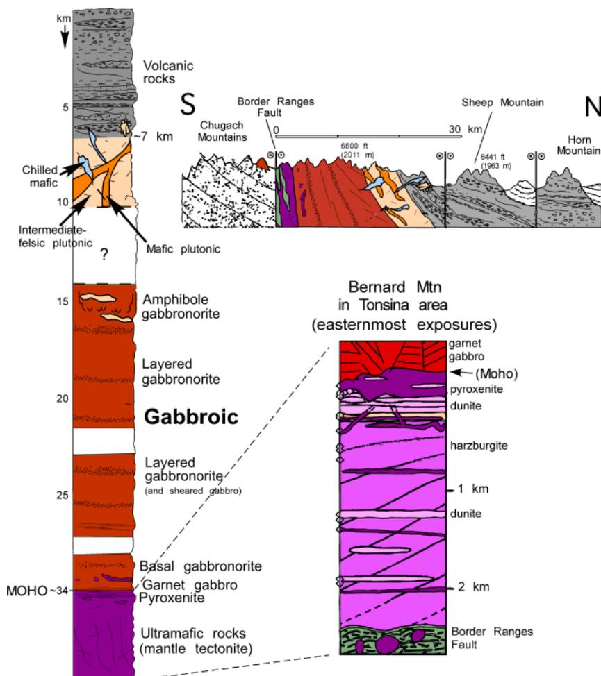
Figure 3. Detailed crustal section for the Talkeetna arc based on stratigraphic thickness of the volcanic section (Clift *et al.* 2005) and geobarometry of Hacker *et al.* (2008). From DeBari and Greene (2011).
