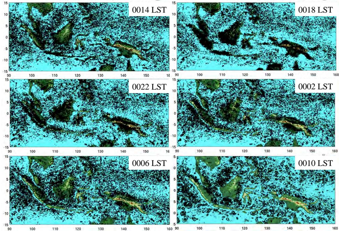
**Figure 2.2** Diurnal cycle of cloud clusters defined as cloud top brightness temperature < 208 K. Sizes of each circle is proportional to the cluster sizes (> 100 km<sup>2</sup>). Courtesy of Shuyi Chen and Brandon Kerns.
