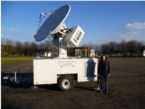
Mobile X-Band Radar Doppler and dual-polarisation capability
